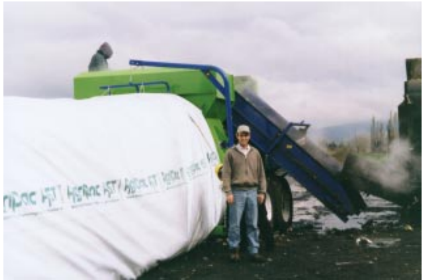
Greg Ryan, General Manager of Z-Best Products in Gilroy, with the conveyor, bagging machine and composting bag used to process material collected from restaurants.
